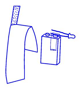
5. Take your paper strip with the duct tape facing down and place the aluminium strip (that was left out of the paper) in a vertical position facing up. With the vertical aluminium strip on the opposite side of the LED wrap the paper strip around the baterry, leaving the LED conector, that isn't glued to the battery, loose. After that, use a piece of duct tape to hold the loose end of the paper.
